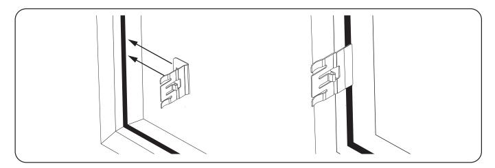
**2.** Fit the bracket by pushing it between the glass and the rubber seal of the window. For ease insertion, use a lubricant in the form of washing up liquid on the base of each bracket. Repeat the proces for each bracket.
