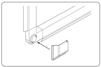
**4.** Turn assembled frame face up and clip supplied Extrusion Corner Covers onto each corner joint.
