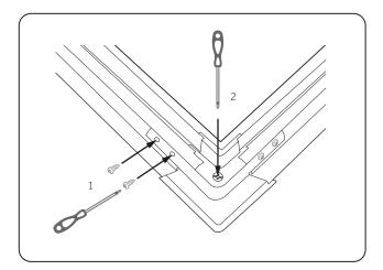
**3.** Secure the side frame components with supplied screws (1) and tighten attached middle corner joint screw (2). Repeat the process for each corner.
