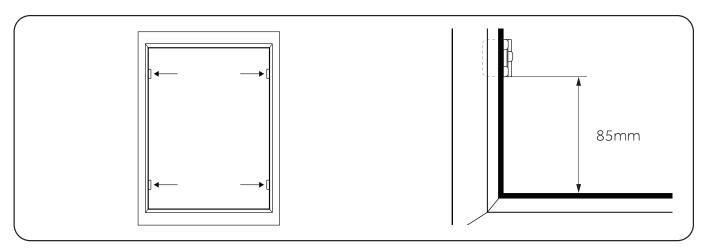
**1.** To ensure all brackets are in correct position for fitting, measure 85mm from top and bottom beading on both sides of the window frame.
