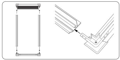
**2.** Guide the side frame components onto the exposed arms of bottom corner joints and follow the same procedure with the top frame compartment.
