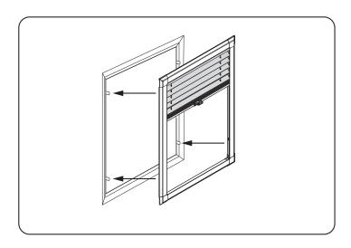
**3.** Clean excess lubricant and clip your Perfect Fit blind onto the window frame.
