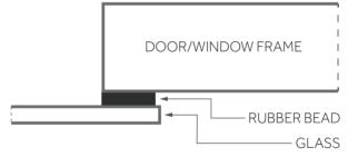
**4.** Using the survey kit, select side profile that best fits the frame. **Ensure that back face of side profile sits flat agaisnt the glass.**
